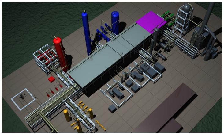
This Fluor Corporation 3D plant model was created in record time by automatically routing pipes.
